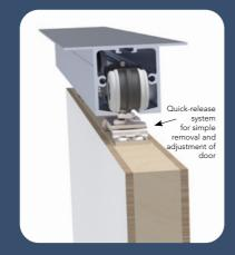
beautiful in its simplicity. The Hallmark Classic is a robust slider unit with a quick-release system allowing the door to be easily removed from the wheel carriage & track. The hanging bracket is hidden from view behind trims or architraves.
