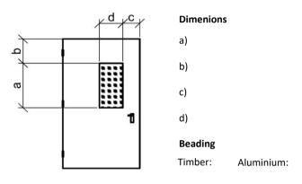
Note: sizes shown refer to Clear View. For Fire Doors, minimum b) dimension must be 200mm and minimum c) dimension must be 150mm. Fire Doors rated FRR-/90/-sm and above can only have VP a) dimension 600mm and b) dimension 100mm with Steel beading
